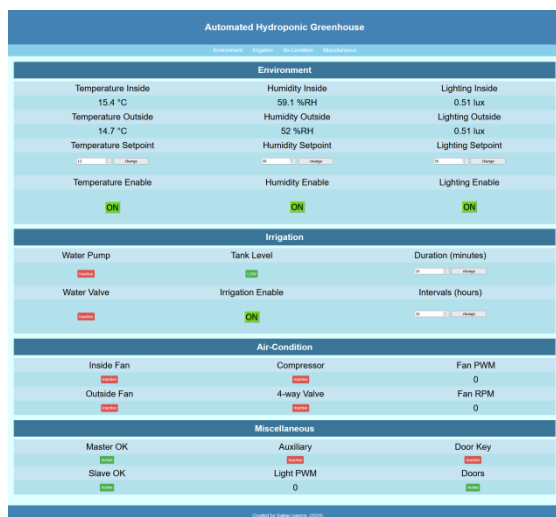
Fig. 7: Remote supervision and control website.
