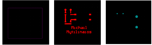
Figure 3. PCB Design in Altium (Cutout, Engrave, Drill).
