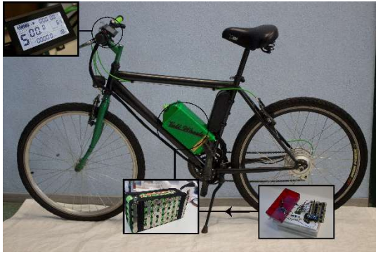
Fig. 1. Battery system components and their spatial placing on the e-bike.
