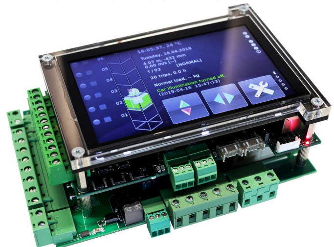
Fig. 4. NOUS Lift Control Board
