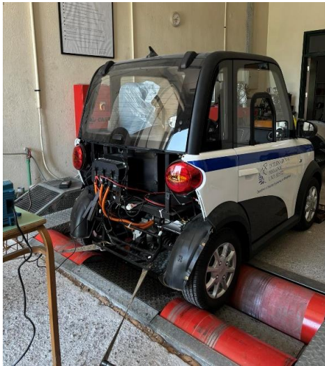
Fig. 1. Electric vehicle secured on chassis dynamometer.
