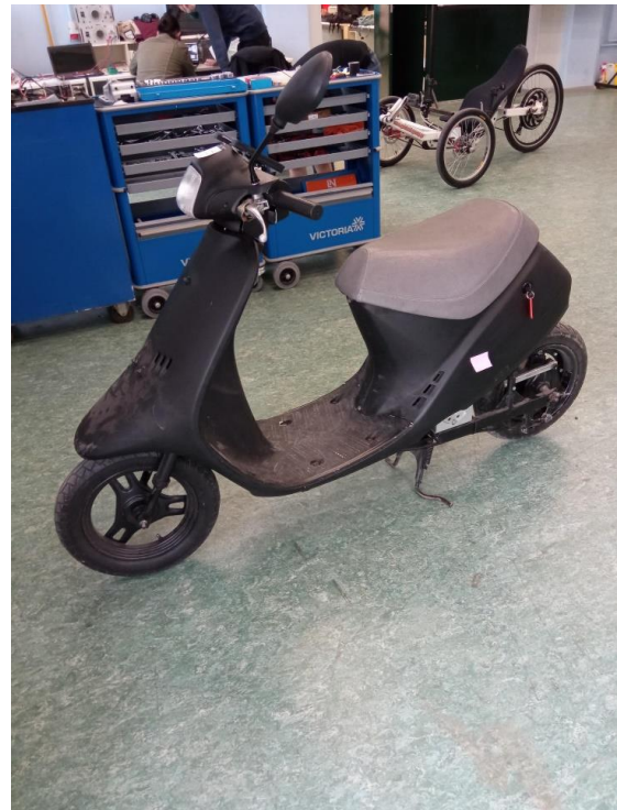
Fig. 1. Yamaha JOG equipped with a 2-stroke single cylinder gasoline internal combustion engine of 50cc.
