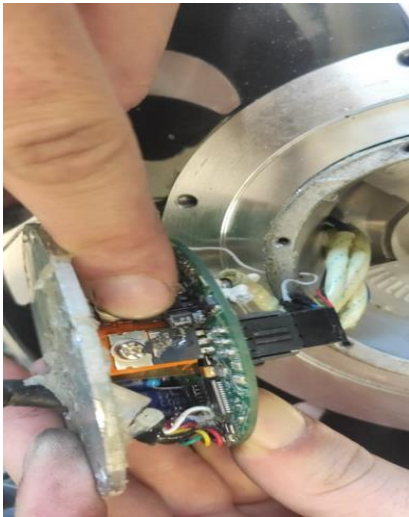
Fig. 2. Picture with defective transistor found inside the wheel motor.
