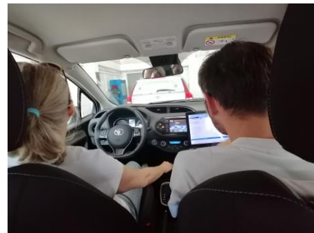
Fig. 6. Data collection process in which the hybrid vehicle is driven while a computer is connected to the vehicle with the Bosch KTS 570 diagnostic tool.
