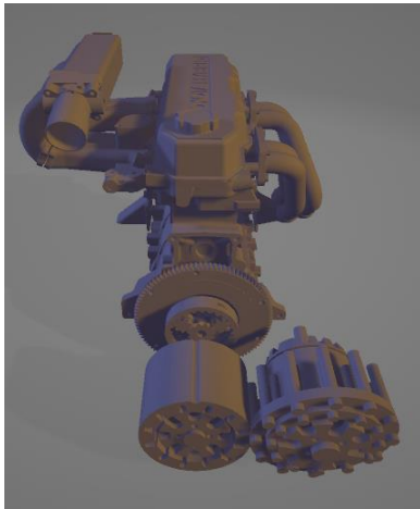
Fig. 7. The 1NZFXE combined engine 3D design showing the characteristic planetary gear of the power split device of the vehicle and in the front the two alternating current synchronous motors.
