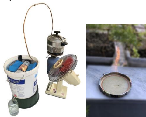
Fig. 4 Distillation and final bioethanol combustion
