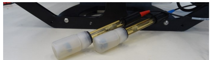
Fig. 1. pH and ORP sensors connected to the ROUV.
