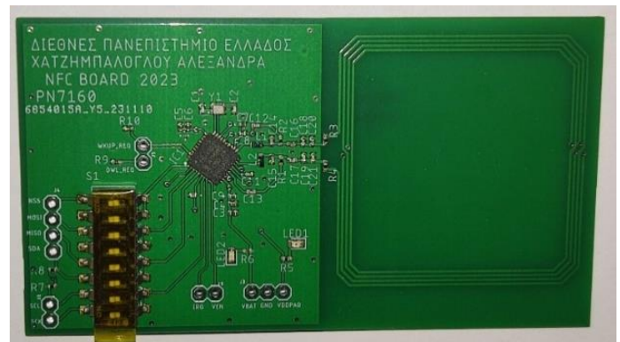
Fig. 4: Top layer assembled board.
